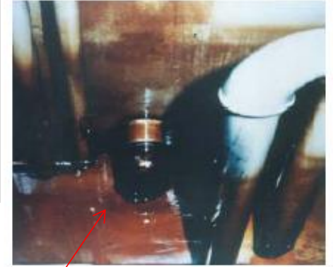
varnish on bearing bush
