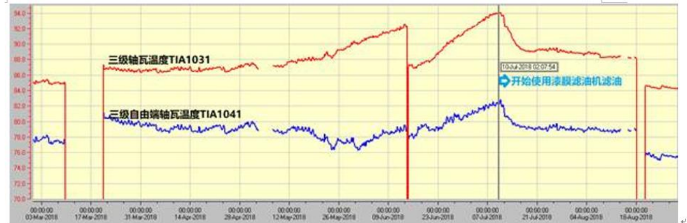
bearing bush temperature trend
